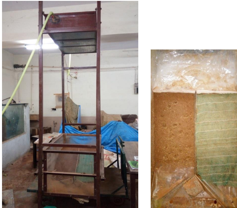
Fig. 5 Industry (M/s Geosol Associates) Sponsored Research Project on Embankment erosion control (Rainfall simulator and embankment model without and with protection)
