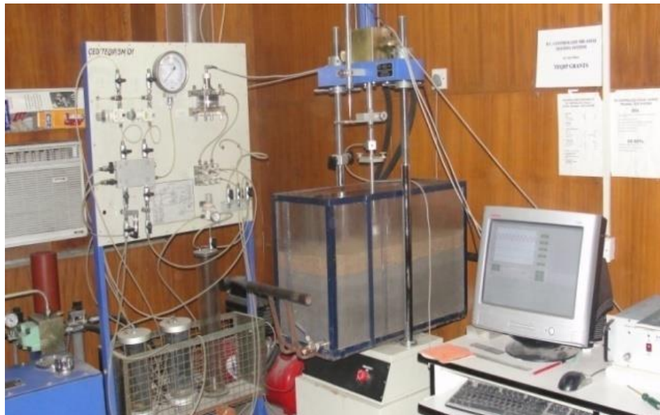
Fig. 2 The PC Controlled Cyclic Triaxial converted in to Cyclic Load Test Facility
